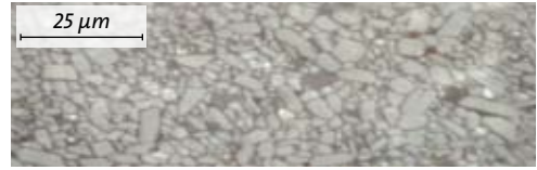
Fig. 3.4: Micrograph showing etched surface of alumina
