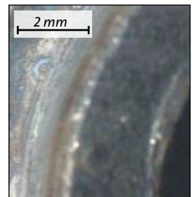
Fig. 5.9: Selective corrosion in cemented tungsten carbide. The metallic binder phase is corroded resulting in reduced wear resistance
