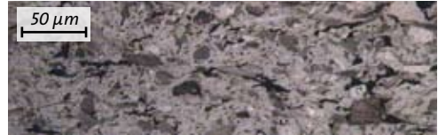
Fig. 3.2: Micrograph showing the material structure of resin-impregnated carbon graphite
