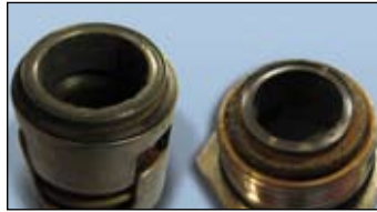
Fig. 5.12: Deep seal face grooves close to the pumped medium side
