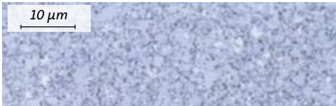
Fig. 3.5: Micrograph showing surface of tungsten carbide
