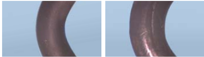
Fig. 5.8: A fresh EPDM O-ring (left) and a swollen EPDM O-ring (right) exposed to water containing mineral oil
