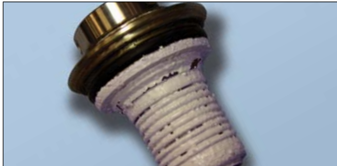
Fig. 5.7: Metal bellows seal clogged by lime scale build-up
