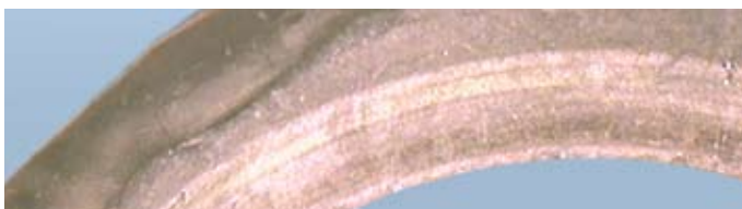
Fig. 5.10: Corrosion of the binder phase followed by severe erosion on a tungsten carbide seal ring with cobalt binder phase
