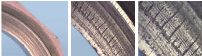
Fig. 5.4: Severe thermal cracks in WC seal face caused by poor lubrication
