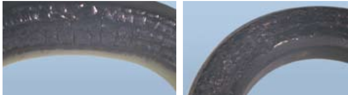
Fig. 5.3: Surface damage due to high temperature on EPDM and FKM secondary seals
