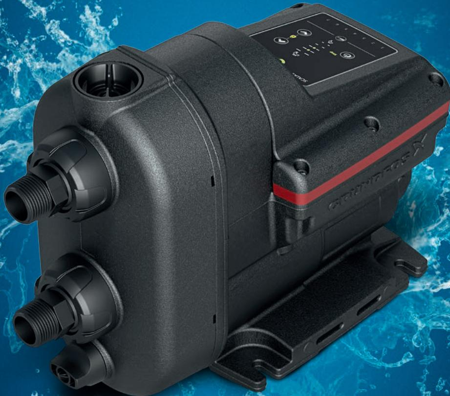
GRUNDFOS SCALA2 is a fully integrated water booster pump delivering perfect water pressure to all taps. It features pump, motor, tank, sensor, drive and non-return valve in one compact unit that installs quickly and easily. With its intelligent pump control, SCALA2 adjusts performance to any demand – and with its water-cooled motor, it offers one of the lowest noise levels in its class. The result is maximum comfort with minimum effort.
