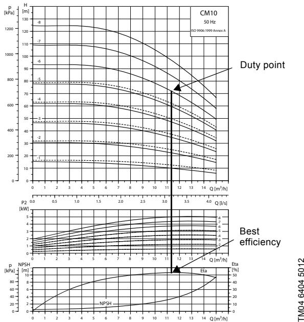
**Fig. 29** Example of a CM pump's duty point
