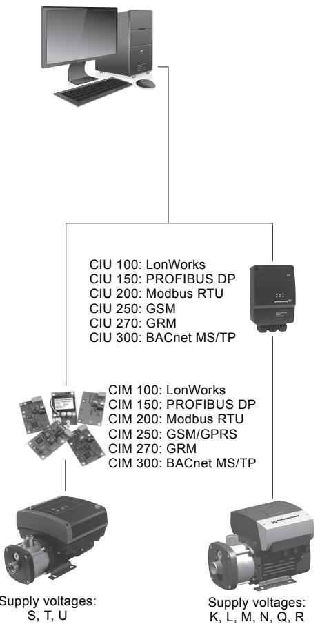
**Fig. 19** Communication via a central building management system
