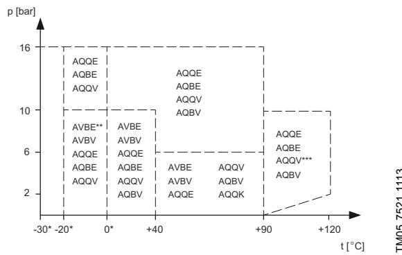
**Fig. 13** Curve for the selection of shaft seals
