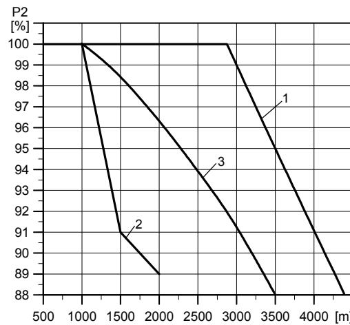
Fig. 10 Relationship between motor output (P<sub>2</sub>) and altitude
