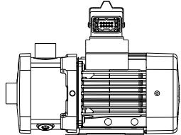
Fig. 34 Motor with multiplug connection
