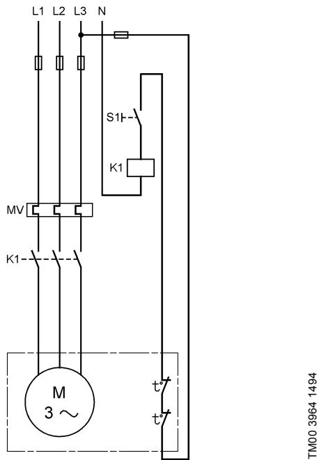
**Fig. 46** Three-phase motor with thermal switches
