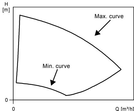
Fig. 22 Min. and max. performance curves
