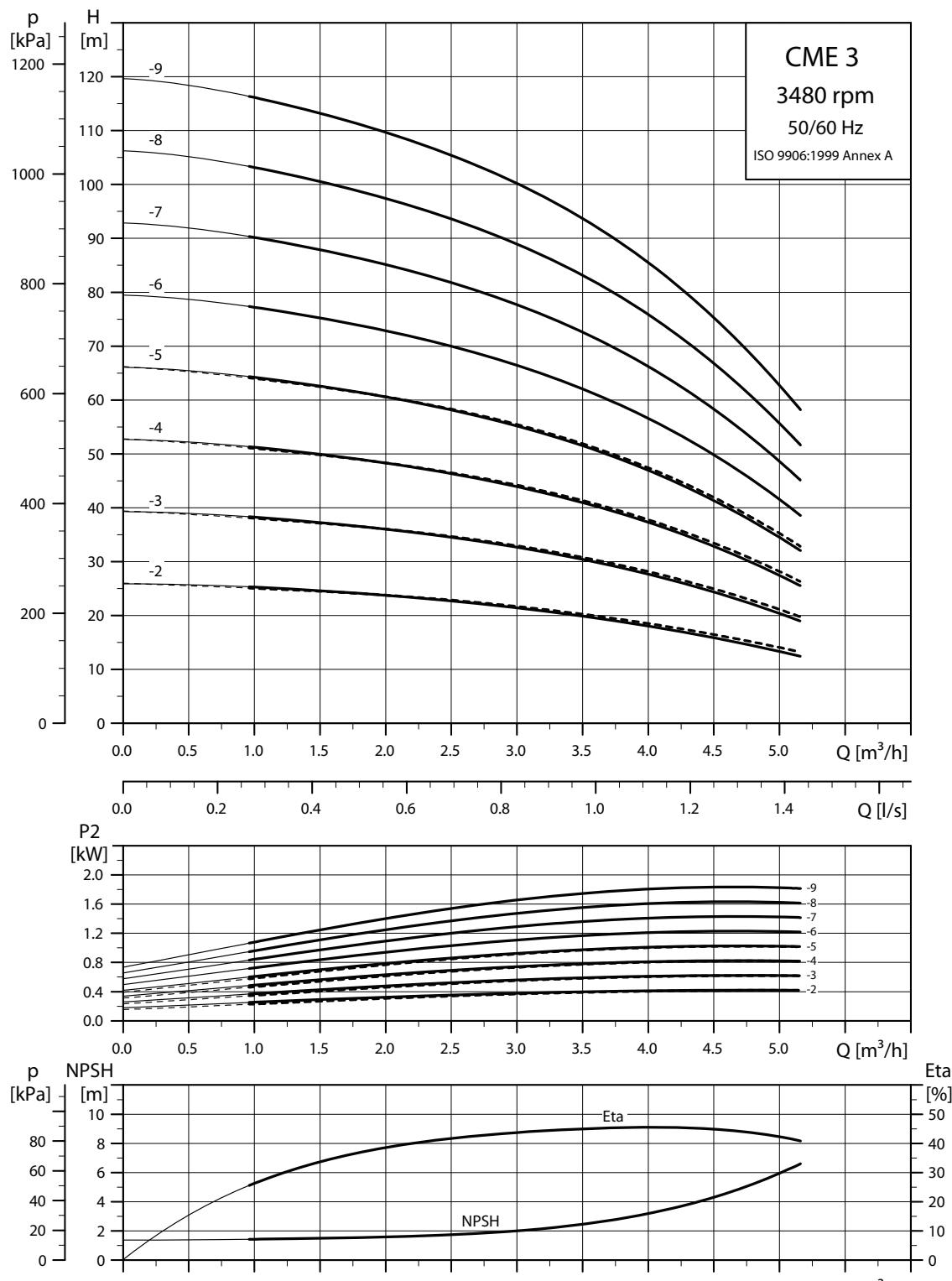
**Note:** Irrespective of the input frequency, the 100 % speed of CME pumps is approximately  $3400 \text{ min}^{-1}$ .
