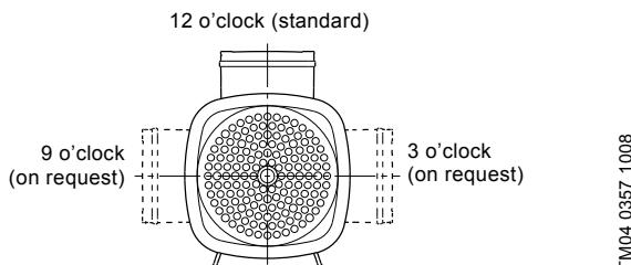
**Fig. 47** Terminal box positions of frame sizes 71 and 80
