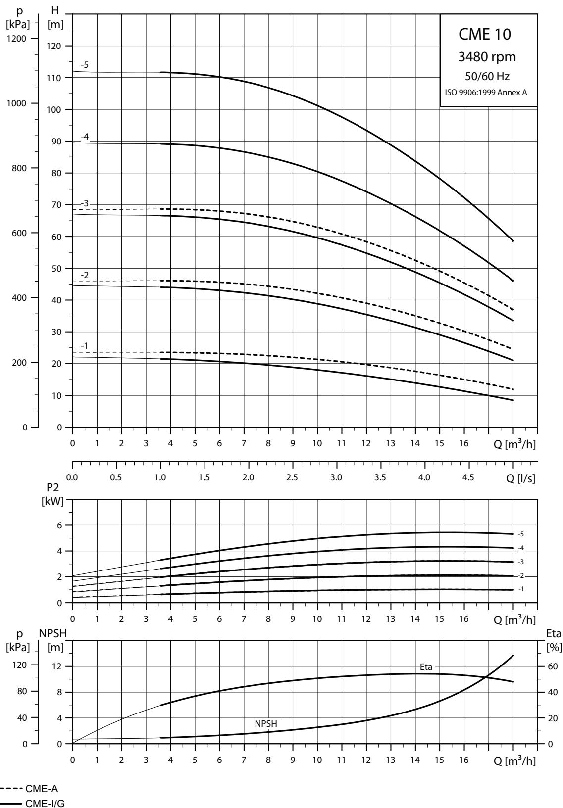
**Note:** Irrespective of the input frequency, the 100 % speed of CME pumps is approximately 3400 min<sup>-1</sup>.
